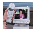
the control board. The color camera doesn't just add value to the AE-500; it adds security to any installation. You can add a CPDM-1 to combine the video signal with an existing CATV network. This will allow all tenants in a development to view on their TVs, who is calling them from the AE-500.
